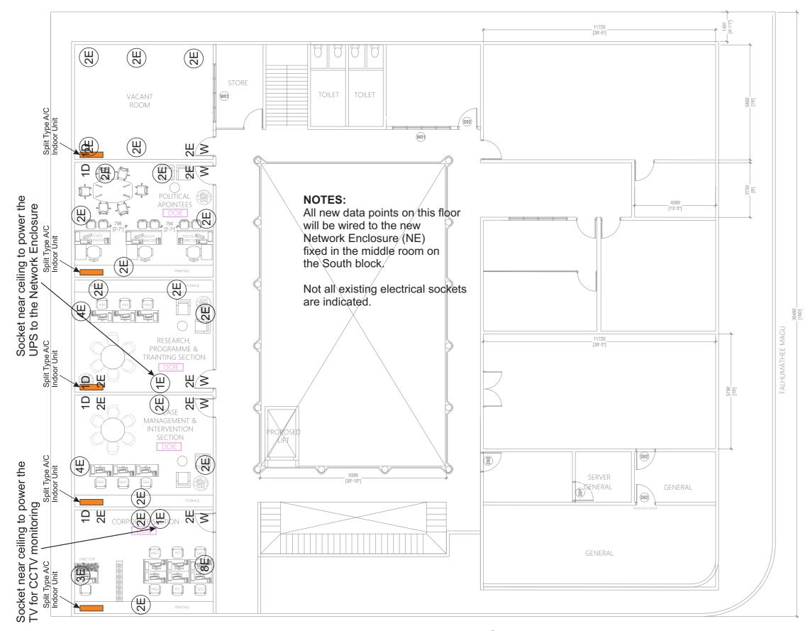
All new power sockets are to be 13 Amperes, UK or Universal type, to be fixed on the walls, 300mm above finished floor level, except for the power socket for the Network Enclosure which needs to be near the ceiling.
